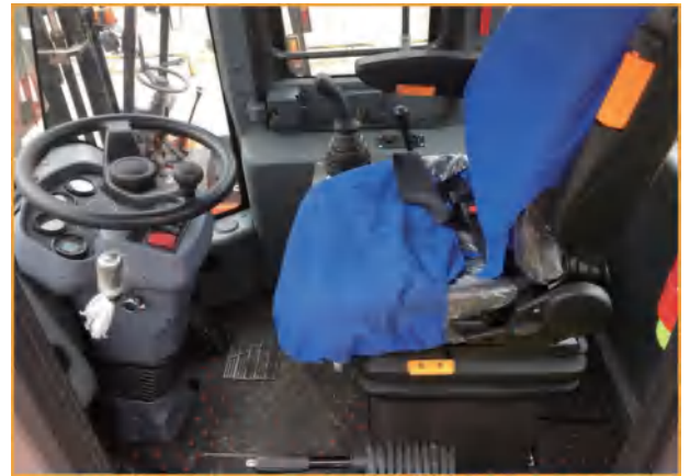
ZL936 CABIN-Hydraulic pilot joystick type
